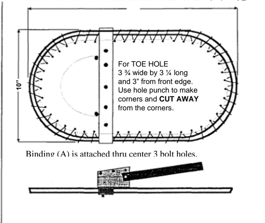
Binding (A) is attached thru center 3 bolt holes.
